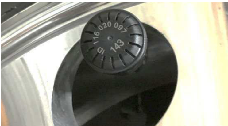
Valve stem mounted tire pressure sensor
