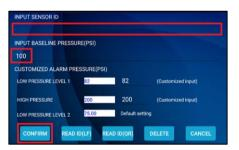
Input the sensor ID#, baseline pressure & alarm levels.
