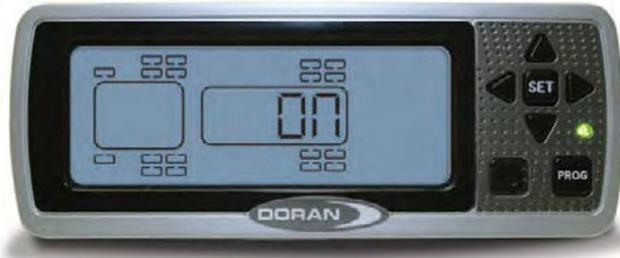
1. With power supplied to the monitor, **PRESS** and **HOLD** the **PROG** button for approximately 5 seconds to enter into **PROGRAM** mode.
