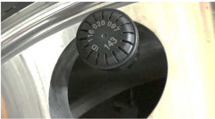
Valve stem mounted tire pressure sensor
