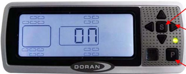
“S” is used to lock in selections during programming. Used to turn on and off the backlight.
