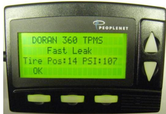
This collaboration between companies will help fleets proactively manage issues that develop from low tire pressures and will help to reduce fleet maintenance costs by providing real-time tire pressure data, warnings and reports directly to the maintenance professionals, in addition to the drivers.
