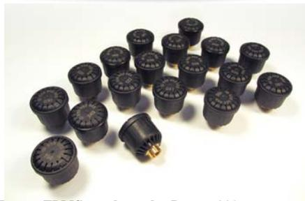
Direct TPMS, such as the Doran 360 series, uses pressure sensors located on each wheel's valve stems to directly measure the pressure in each tire. These sensors broadcast pressure data via a wireless radio frequency transmitter to a central receiver where the data is analyzed and the results sent to a display mounted inside the vehicle.
