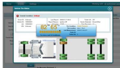
DRILLDOWN ON SPECIFIC VEHICLE WITH CURRENT PRESSURE/TEMPERATURE AND HISTORICAL DATA
