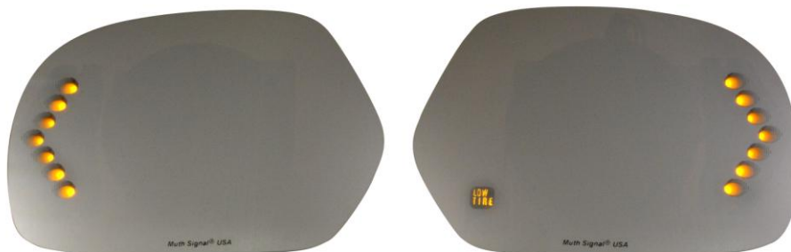
Muth Mirror Signal Unit Honda Gold Wing (Chrome Glass/Amber Light) with “LOW TIRE” indicator
