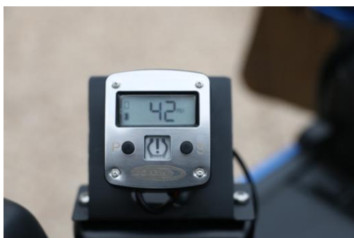
Doran 360M™ tire pressure monitoring system: monitor/display
