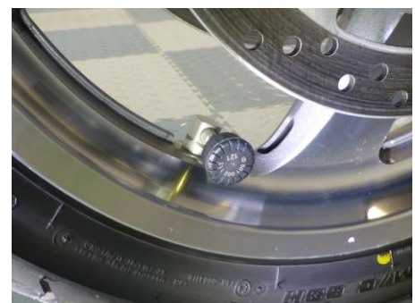
Doran 360M™ tire pressure sensor
