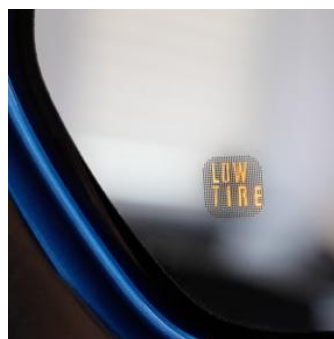
Muth Mirror Signal Unit “LOW TIRE” LED indicator
