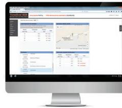
A customer-specific secured web portal can be accessed to see current and historical tire pressure/temperature data and alarms. The portal may be configured to send alerts via text message (SMS) or email to multiple recipients. Cloud storage and portal access require a contract and payment for data/hosting fees.
