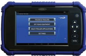
The Doran SmartLink™ TPMS tablet is used to program Equipment ID# and tire pressure sensor information to the Doran TPMS Hub.
